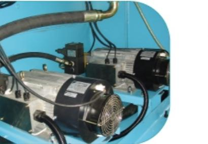
The large capacity machine is equipped with several sets of power saving servo pumps (Japan imported).
