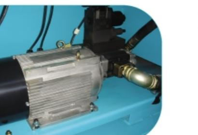
The servo motor employs an encoder and pressure sensor for fully closed-loop control of oil flow and pressure.
